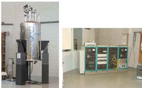
Figure 1.6. A 14.1 Tesla superconducting magnet (equivalent with 600 MHz for ^1\text{H} -NMR) placed in the Goudsmit Pavilion in Nijmegen (left), together with the console containing the necessary electronics for NMR spectroscopy (right).
